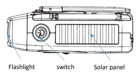
The radio can be fully charged after 66 hours by placing it in the direct sunlight.
